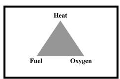
If the sides of the triangle are not allowed to meet – if the triangle does not form, there will be no fire.
